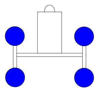
If one vacuum circuit develops a leak, for example when a vacuum line gets severed, the load drops because the suction cups are no longer able to carry anything.
