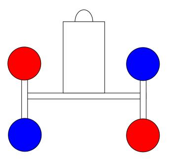
On a properly configured 2-circuit vacuum lifting device, if a vacuum hose gets severed, nothing affects a nominal rating. It remains supported by the suction cups. However, a visual and/or acoustic warning should be issued. In addition, the affected vacuum control meter should display the danger area.
